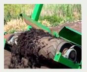
Machinery turns and mixes the piles, incorporating air that helps in the decomposition process. Temperature and moisture are carefully monitored, ensuring that the natural process can unfold regardless of weather conditions.
